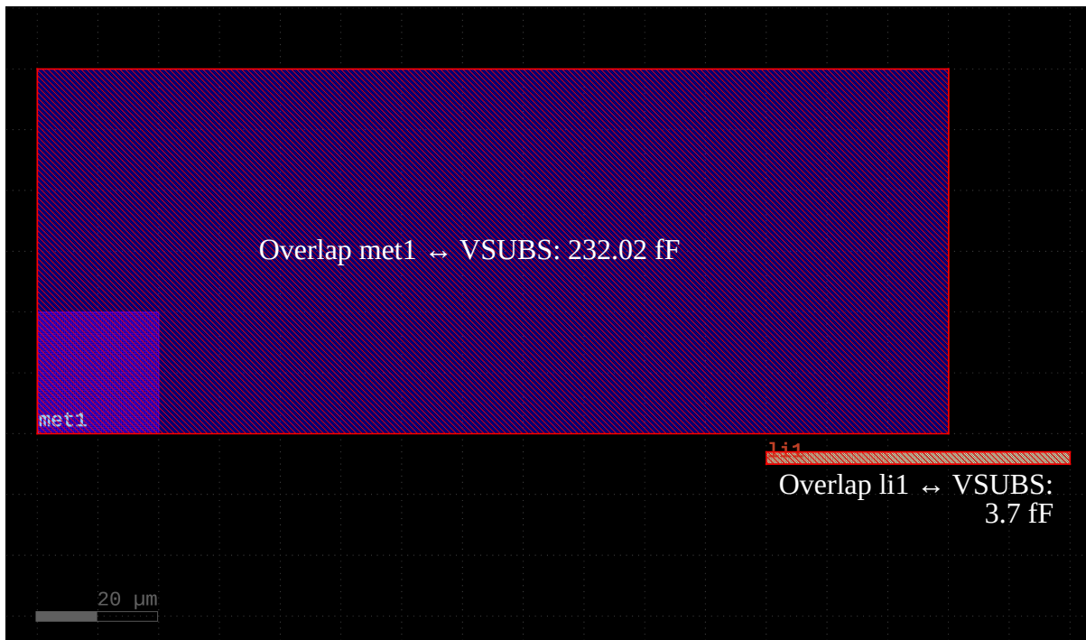
Figure 23: Overlap capacitances to substrate.
